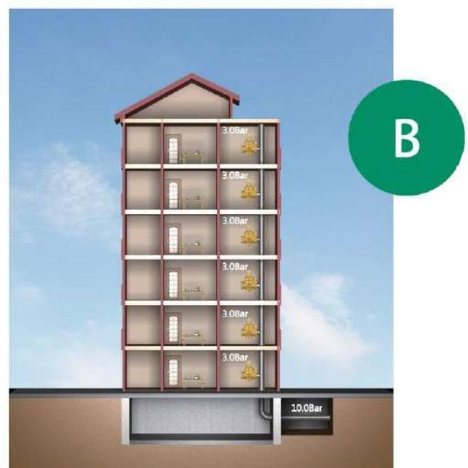
For buildings with more than 5 floors, pressure reducing valves must be installed in each home or floor to make sure that all the floors have the same inlet pressure. In this case, it's also advisable to install a bigger pressure reducing valve in the main inlet pipeline of the building.
