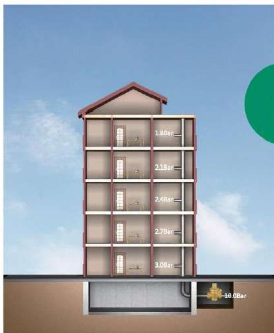
For buildings with equal or less than 5 floors, pressure reducing valve can be installed in the main inlet pipeline. This produces a pressure differential in each floor. As example, if the height between each floor is 3m, every each floor higher, the pressure reduces 0,3 bar.
